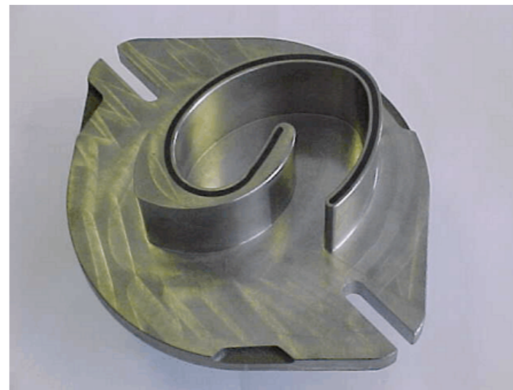
Figure 4 Moving scroll V1.0
